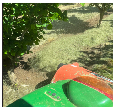
Side-discharging grass clippings onto hazelnut rows with prototype mower.
